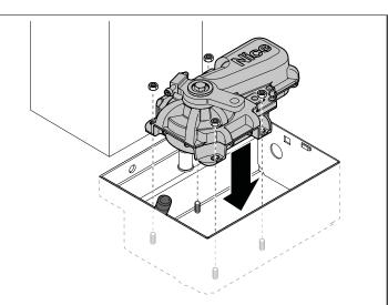
**05.** Mount the control bracket on the box's stud along with the ball
