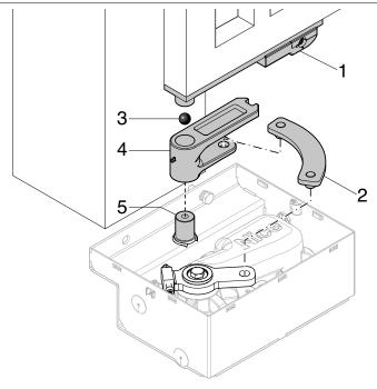
**06.** Place the gate leaf on the release lever and secure it with bolts (a) or a strong weld (b)
